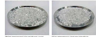
(Before measurement) The sample was spread evenly over the pan. (After measurement) There was basically no change in appearance.
